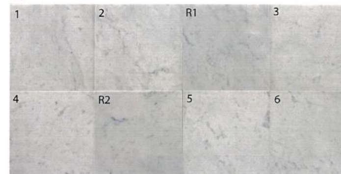
Figure 1b. Test specimens after the exposure, including two reference specimens that are not exposed.
