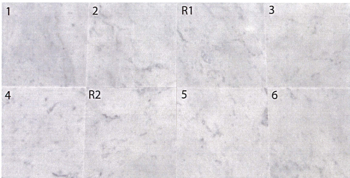
Figure 1b. Test specimens after the exposure, including two reference specimens that are not exposed.
